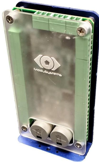
The BLC-2T is a Dual Axis Modular Stepper Motor Controller with Integrated Amplifiers.
