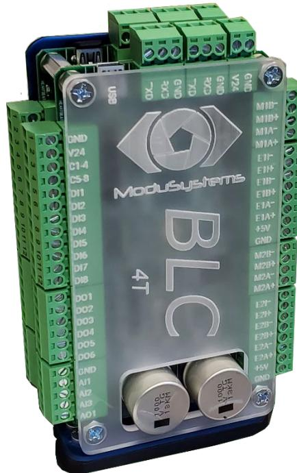
The BLC-4T is a 4 Axis Modular Stepper Motor Controller with Integrated Amplifiers.
