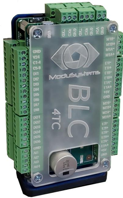
The BLC-2TC is a 4 Axis Modular Controller for controlling 2 Digital Servo Drives or 2 External Stepper Drives.
