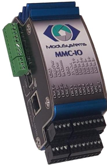
The MMC-IO is a Modular I/O Control Module that can be combined with any other MMC Controller to add I/O resources. High Speed Differential Inputs and Outputs can allow for control of additional On/Off or Frequency Controlled Devices.
