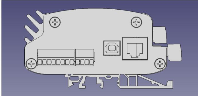
Clearance required for right side connector. Ensure clearance is provided for airflow around heat sink fins when operating at higher current levels. Avoid mounting controller inverted as this traps air in the heat sink fins. Insure clearance on left side for wiring, USB, and Ethernet connectors.
